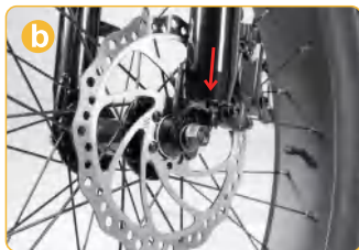
b. Sit the front fork on the axle of the front wheel.
